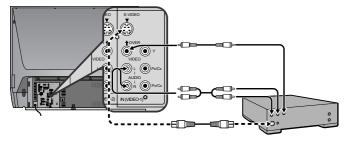
Note that the connection with a video cable will be ignored in case you connect a VCR to the TV with both video cable and S-VIDEO cable.
