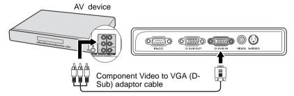
If the selected video image is not displayed after the projector is turned on and the correct video source has been selected, check that the Video source device is turned on and operating correctly. Also check that the signal cables have been connected correctly.
