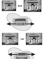
Then sharpen the image by rotating the focus ring.
