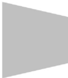
From the projector, the image path is shorter along the right side.
