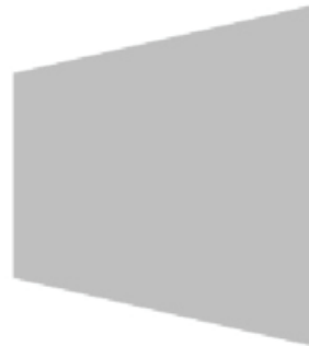
From the projector mirror, the image path is shorter across the right side
