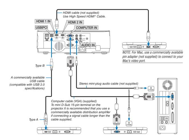
Select the source name for its appropriate input terminal after turning on the projector.
