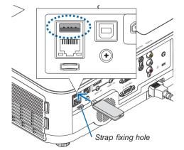
To remove the USB Wireless LAN Unit, disconnect the power cord and use the above procedure.
