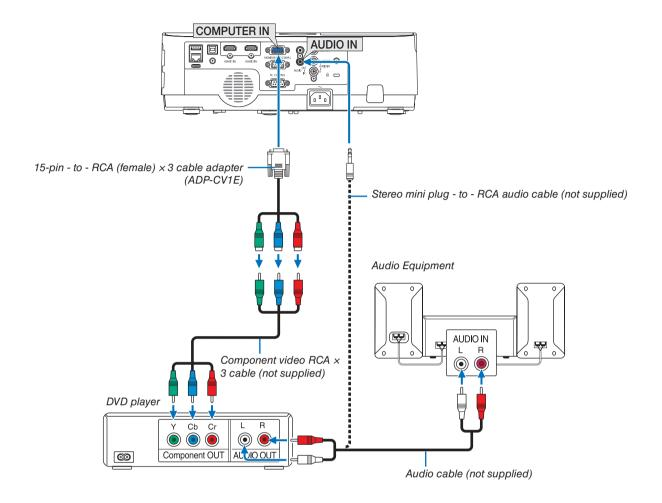
A component signal will be automatically displayed. If not, from the menu, select [SETUP]  $\rightarrow$  [OPTIONS(1)]  $\rightarrow$  [SIGNAL SELECT]  $\rightarrow$  [COMPUTER], and then place a check mark in the Component radio button.
