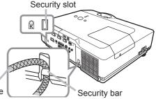
$\triangle$  **WARNING**  $\triangleright$  Do not use the security bar and slot to prevent the projector from falling down, since it is not designed for it.
