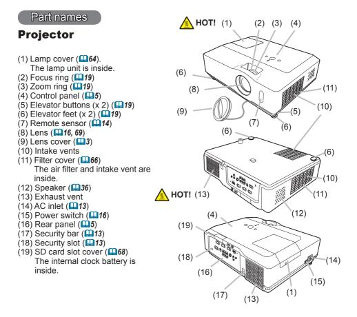
▲ **WARNING** ► HOT! : Do not touch around the lamp cover and the exhaust vents during use or just after use, since it is too hot.
