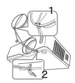
2. Fix the strap to the strap hole of the projector.
