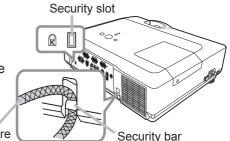
**△WARNING** ► Do not use the security bar and slot to prevent the projector from falling down, since it is not designed for it.
