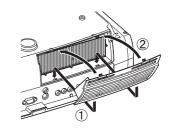
3 Loosen the lamp fixing screws.
