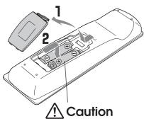
Check the (+) and (-) indications inside the battery compartment and insert the batteries so that they face correctly. At the time of purchase, the batteries are not inserted into the remote control. Insert the supplied batteries before using the remote control.
