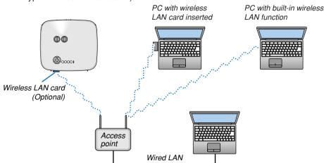
To make connection with a wired LAN via an access point, you need to select the Infrastructure mode. From the menu, select [Setup]  $\rightarrow$  [Installation]  $\rightarrow$  [LAN Mode]  $\rightarrow$  [PC Card]  $\rightarrow$  [Advanced]  $\rightarrow$  [Network Type]  $\rightarrow$  [Mode]  $\rightarrow$  [Infrastructure].
