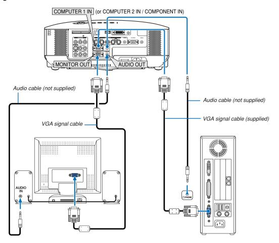
You can connect a separate, external monitor to your projector to simultaneously view on a monitor the RGB analog or component image you're projecting.
