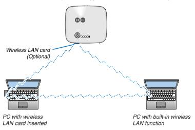
To enable direct communication (i.e., peer-to-peer) between personal computers and projectors, you need to select the 802.11 Ad Hoc mode.
