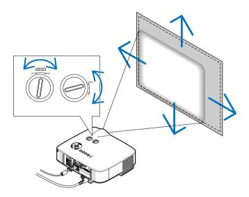
NOTE: The lens shift dial for LEFT-RIGHT cannot be rotated one-half turn or more. Do not over rotate it or it may break.
