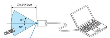
Remote sensor on the remote mouse receiver
