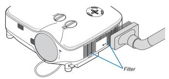
To reset the filter usage time, from the menu, select [Reset]  $\rightarrow$  [Clear Filter Hours]. ( $\rightarrow$  page 107 for resetting the filter usage time)
