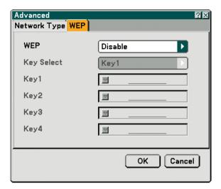
Select this option whether using the WEP (Wired Equivalent Privacy) key for encryption or not. To use encryption, specify WEP key.
