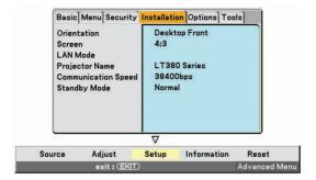
5 Press the SELECT ▼ button three times to highlight "LAN Mode", and press the ENTER button.
