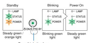
Press this button for a minimum of 2 seconds.
