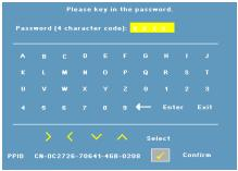
CHANGE PASSWORD—Allows you to change the password. Key in the original password and then enter the new password. Enter the new password again to confirm.
