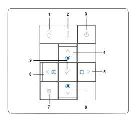
LAMP warning light If the LAMP light is solid amber, replace the lamp. If the LAMP light is blinking amber, the projector automatically shuts down indicating a system failure. If this problem persists, contact Dell.
