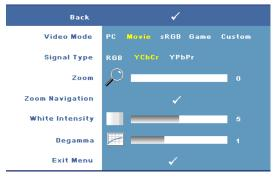
VIDEO MODE—Select a mode to optimize the display on how the projector is being used: PC, Movie, sRGB (provides more accurate color representation), Game, and Custom (set your preferred settings). If you adjust the settings for White Intensity or Degamma, the projector
