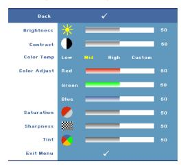
**Brightness**—Use  $\triangleleft$  or  $\triangleleft$  to adjust the brightness of the image.
