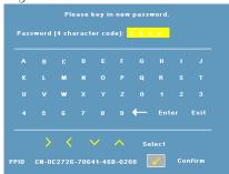
Enable the Password function will pop-up a character screen, key in a 4digit number from the screen and press the Enter button.
