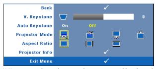
**V. KEYSTONE**—Adjusts the image distortion caused by tilting the projector.
