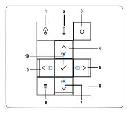
1 LAMP warning light If the LAMP light is solid amber, replace the lamp. If the LAMP light is blinking amber, the lamp driver or color wheel have failed and the projector automatically shuts down. If the problem persists, contact Dell<sup>™</sup>.
