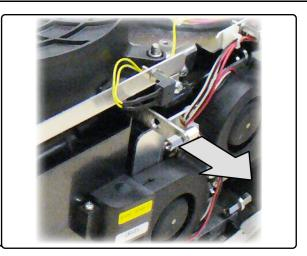
Image 3-8 Lamp 1 locking system must be unlocked
