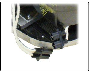
Image 3-11 Lamp 1: make the power connection
