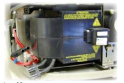
Image 3-9 disconnected lamp connector
