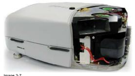
Image 3-7 right view of the projector, rear cover removed
