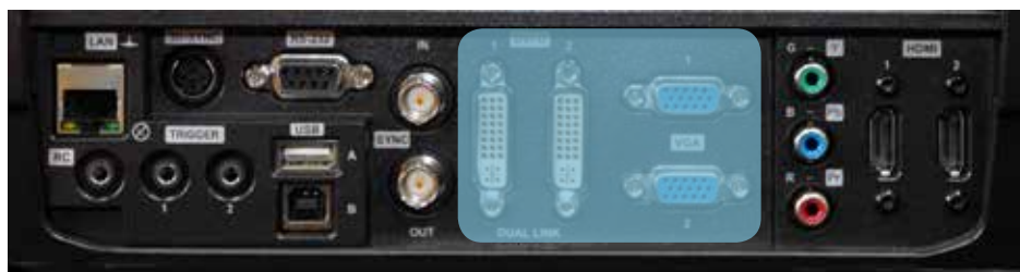
Figure 5-5. Connecting a computer source
