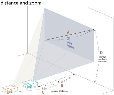
The table below shows how to achieve a desired image size by adjusting either the position or the zoom ring. For example: to obtain an image size of 50" set the projector at a distance 1.6 m and 1.9 m from the screen and adjust the zoom level accordingly.
