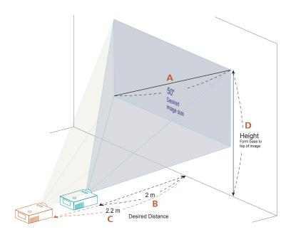
The table below shows how to achieve a desired image size by adjusting either the position or the zoom ring. For example: to obtain an image size of 50" set the projector at a distance 2 m and 2.2 m from the screen and adjust the zoom level accordingly.
