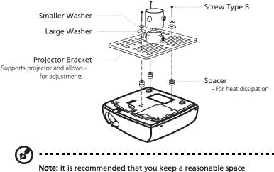
**Note:** It is recommended that you keep a reasonable space between the bracket and the projector to allow for proper heat distribution. Use two washers for extra support, if deemed necessary.
