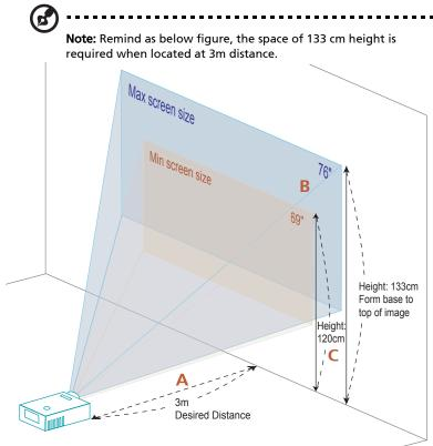
Figure: Fixed distance with different zoom and screen size.
