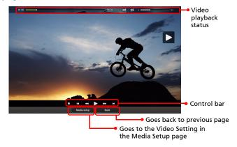
You can press ◀/▶ to adjust the volume. To select the backward/forward speed, press the Rewind/Fast-forward key repeatedly. To display the subtitle, you can press A/a on the remote control (if available) to trigger the projector OSD subtitle menu. For details on the Video Setting, see "Video Setting".
