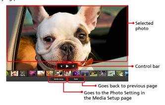
You can press ▶ to start a slideshow in full screen. Music playback is allowed during a slideshow. You can press ◀/▶ to adjust the volume. For details on the Photo Setting, see "Photo Setting".
