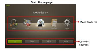
This mode allows you to browse media files stored in different devices, such as RAM (internal memory), USB handy drive, USB hard drive and SD card (for selected models) when connected to the projector. No matter where you are, you can always press MEDIA HOME to go back to MEDIA HOME page.
