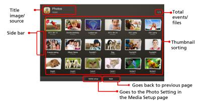
You can press the four directional selection keys to select the file and press ENTER to access. To use the side bar, press ◀ repeatedly until it displays and you can browse files by events/photos.
