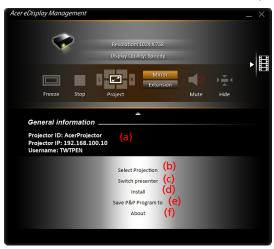
The Main tab of the full UI displays Projector ID, Projector IP and User name information (a), and gives you the option to select a different wireless projector (b). Change other NB/PCs who connected this projector by Switch presenter (c). You may also do real installation in hard disk via P&P token by clicking Install (d) or make another token via Save P&P (Plug & Play) Program to (e). About (f) displays version information of Acer eDisplay Management.
