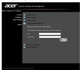
The WPA-PSK/WPA2-PSK encryption key should be entered as 8 to 63 ASCII characters. This feature can be set and enabled by the supervisor.
