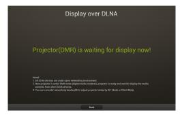
The projector works as a Digital Media Renderer (DMR) and waits for display media content from other DLNA compliant devices under the same local area network. The function works either when the projector is in AP mode or Client mode.
