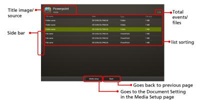
You can press ▲/▼ to select the file and press ENTER to view it. To use the side bar, press ◄ repeatedly until it displays and you can browse files by document file formats. Button operations are different when viewing different types of documents.
