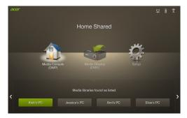
The projector works as a Digital Media Player (DMP) to browse and play media from other DLNA compliant devices or NB/PCs under the same local area network. The function works either when the projector is in AP mode or Client mode.
