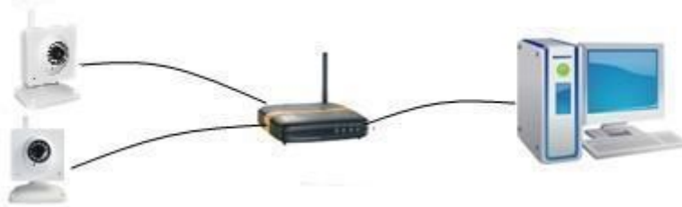
Picture 10 Connection between Several IP camera and router
