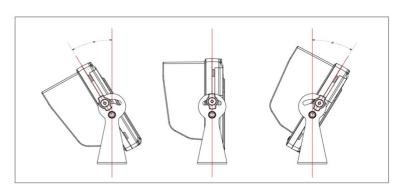
The U-shaped mount stand bracket separates from the LCD display housing for attachment / fixture. The U-shaped bracket attached to the desired location via 3 screw holes located at the base of the bracket. Please remove the LCD display monitor from the bracket before attempting to secure the bracket to your desired location.
