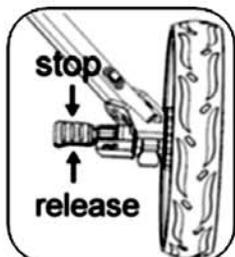
Push down the brake pedal to stop the cart and pull up to release.
