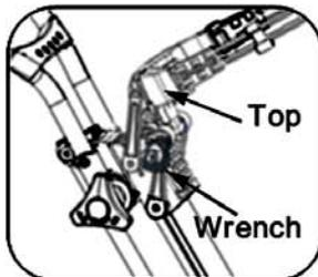
Press the wrench to fix the bracket, and pull up the wrench to adjust the bracket to a proper position.
