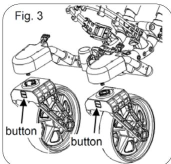
Press the button to assemble front wheel as in fig.3.
