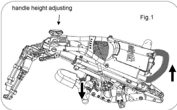
Make sure the handle height adjusting knob is fully tightened.
