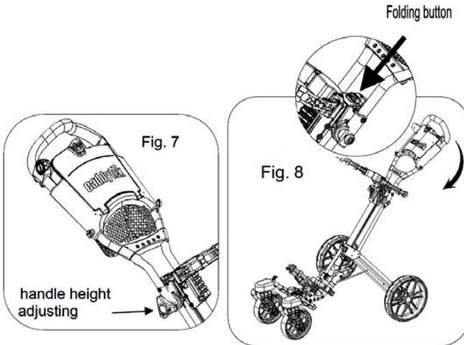
Make sure the handle height adjusting knob is fully tightened. Slightly lift up the handle as Fig. 7 then press the folding button and push the handle downward as shown in Fig. 8 , Fig. 9 to fold the cart till the main frame clicks into the holding slot as in Fig.10 .
